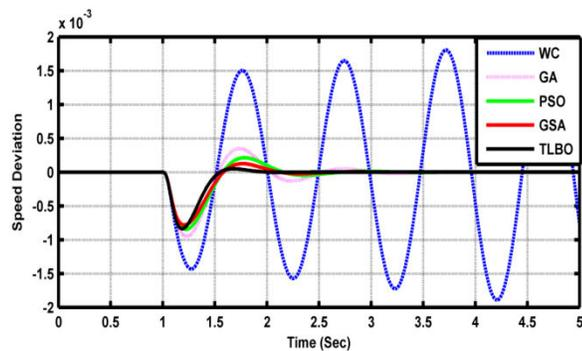
Fig.9 Speed Deviation for 25% Increase in Machine Inertia at (b) condition
