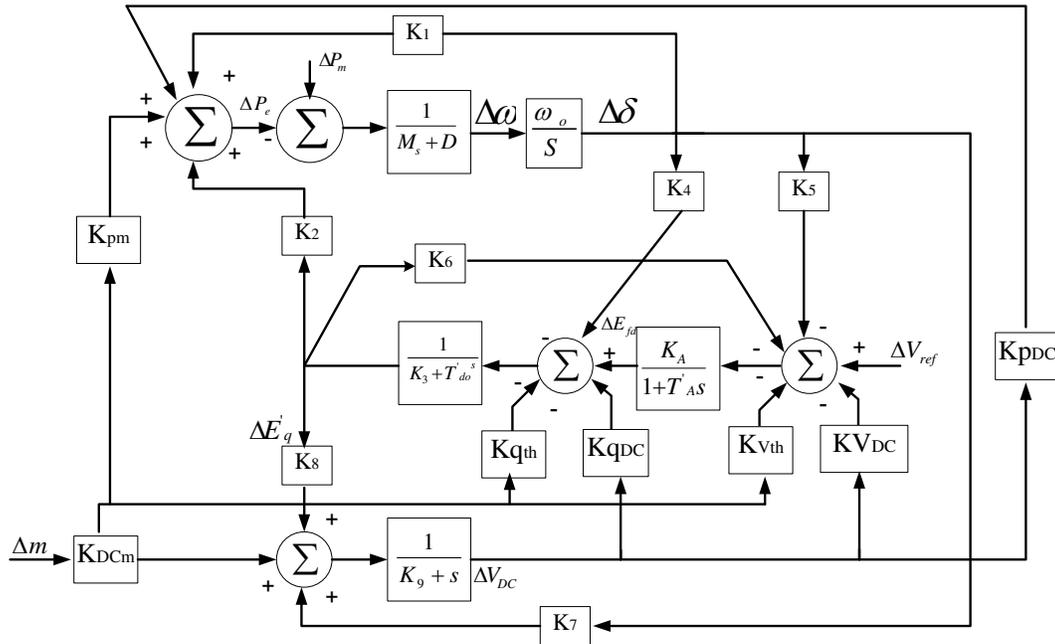
Fig.4 Haffron Model of SMIB with SSSC [7]
