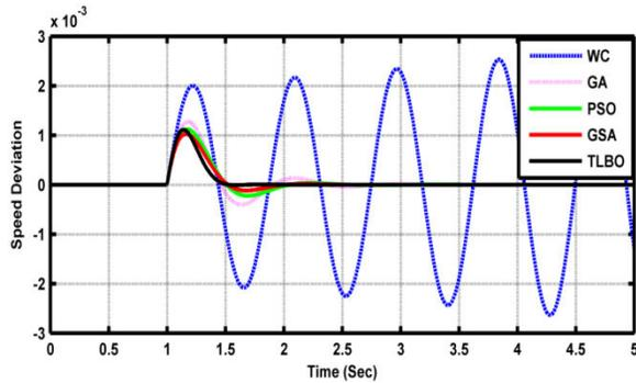
Fig.14 Speed Deviation for 25% Decrease in Direct Axis Time Constant at (a) condition
