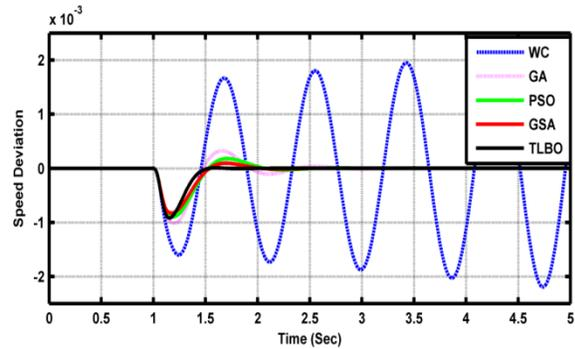
Fig.15 Speed Deviation for 25% Decrease in Direct Axis Time Constant at (b) condition
