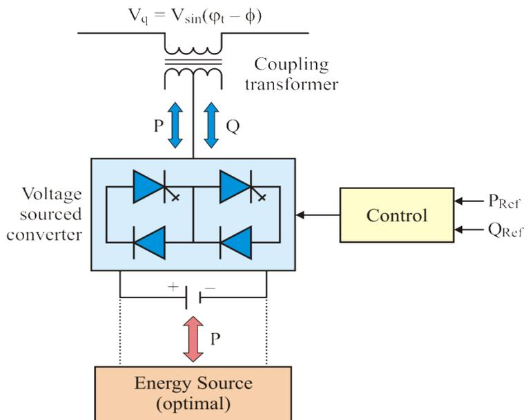
Fig.2: Transmission line with SSSC.
