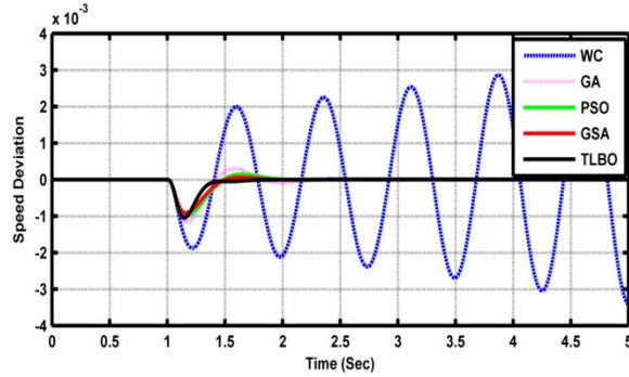
Fig.11 Speed Deviation for 25% Decrease in Machine Inertia at (b) condition
