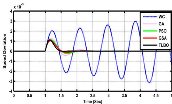
Fig.12 Speed Deviation for 25% Increase in Direct Axis Time Constant at (a) condition
