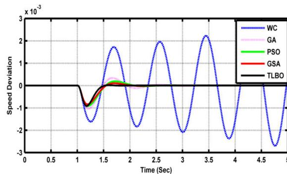
Fig.13 Speed Deviation for 25% Increase in Direct Axis Time Constant at (b) condition
